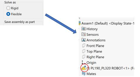
The subassembly icon shows the robot can be manipulated directly in the top-level assembly.
