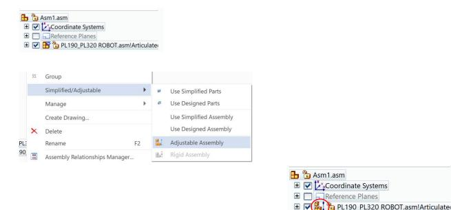
The subassembly icon shows the robot can be manipulated directly in the top-level assembly.
